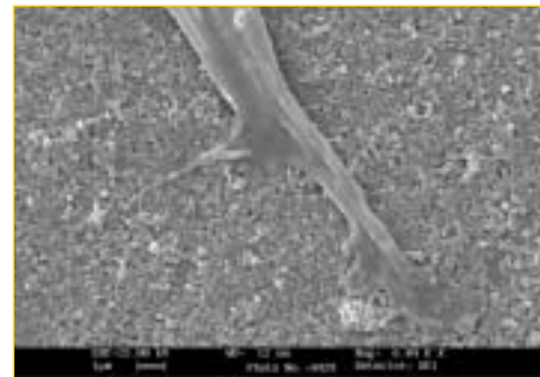
Scanning electron micrograph of contact between a neuron and a carbon nanotube substrate. (Courtesy of Laura Ballerini.)
